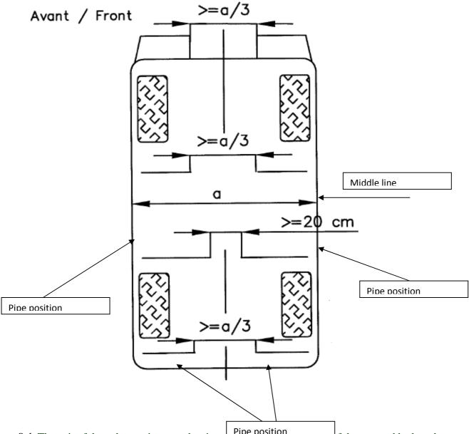
**8.4.** The exit of the exhaust pipe must be situated within the perimeter of the car, and be less than 5 cm from this perimeter.
